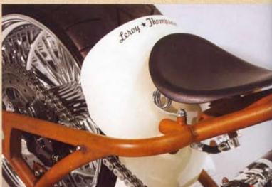
stoplights and operate the kickstand. The Pingel unit even has an ignition interrupt, so you don't have to use the clutch while shifting if you don't want to. The true dirty touch on this bike is the actual copper oxide rusted frame that gives the bike the other half of its name. The process is a controlled chemical oxidation that is done in-house at Leroy-Thompson.
